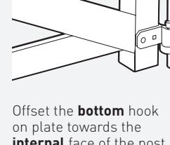
Offset the **bottom** hook on plate towards the **internal** face of the post.
