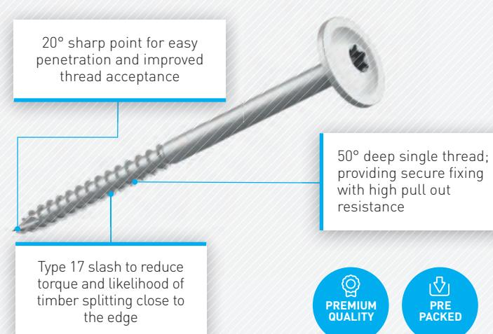
50° deep single thread; providing secure fixing with high pull out resistance
