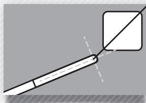
Positioning the gate so the edge is on the corner of the post ensures the gap between the two remains consistent; removing the danger of finger trapping, bringing you in line with legislation.
