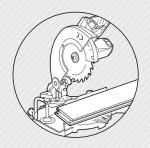
To reduce gate height cut uprights (A/B) down in 150mm increments.
