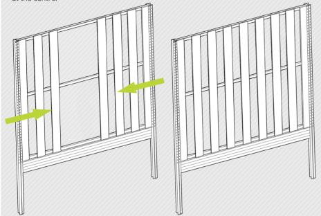
When spacing the boards, it can be helpful to use your adjustable clamps to hold the spacer in place while you fix the top of the board. Then it is easy to use a spirit level to ensure that the board is straight, before fixing the middle and bottom.
