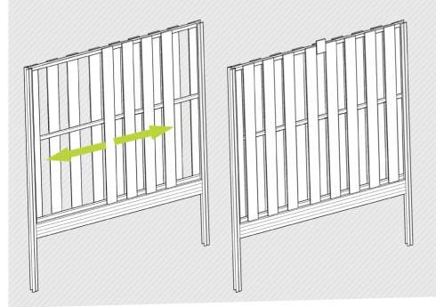
Optimal screw placement: three per board to save time when installing. Alternating the placement in this way allows you to speed up the process and then the rest of the screws can be fixed once the spacing is complete.
