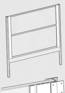
We advise that when doing this step you should begin with the top rail, sandwiching it each side between a 115mm composite board and a 30mm composite board. At this point it is best to use a quick-release clamp to pin the top cross rail in place on one side while you level and fix on the other. The same can then be repeated on the middle and bottom rails.
